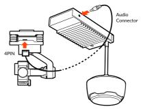
IMPORTANT NOTE: In this User Manual, the TYPHOON is taken as an example. If you have any other compatible power supply equipment or wearable equipment, you can plug the 4PIN power connector of the MK58 into power output port of other equipment as well.
