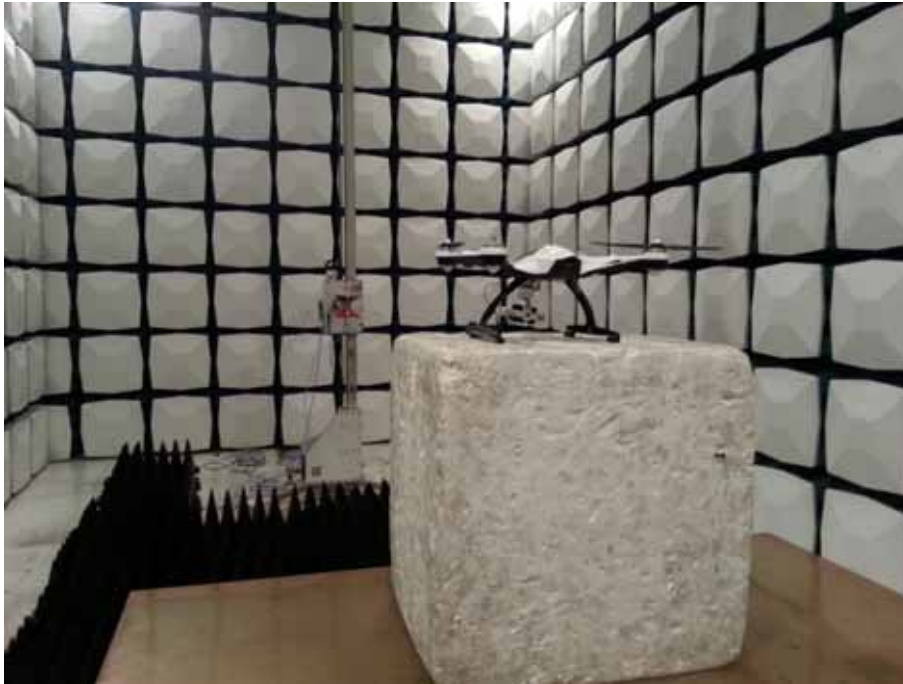
Description: Radiated Emission Test Setup for 1~18GHz
