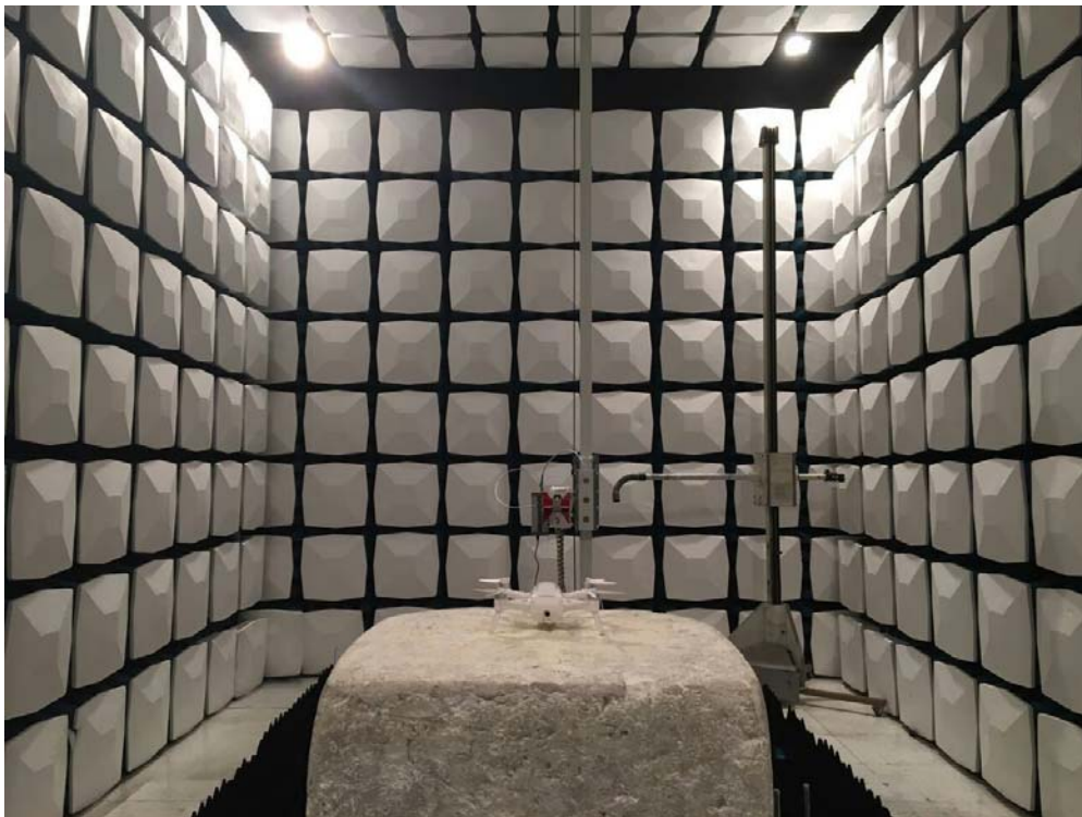
Description: Radiated Emission Test Setup for 1~18GHz
