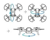
The LED indicator blinks white or yellow during the whole compass calibration process, when you complete the process, the LED will blink green and Breeze will emit an audible sound. Recalibrate the compass if the LED blinks red as this means calibration has failed.
