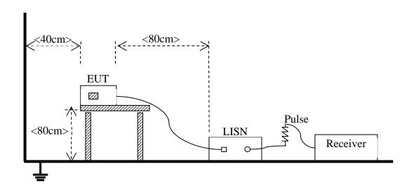
(For Conducted Emission, AC Ports Test)
