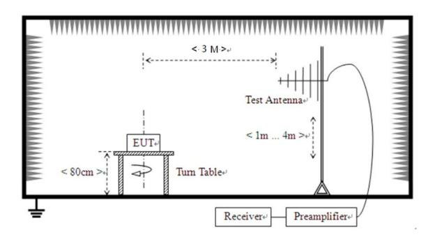
(For Radiated Emission Test (30 MHz-1 GHz))
