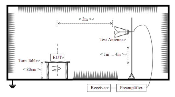
(For Radiated Emission Test (above 1 GHz))
