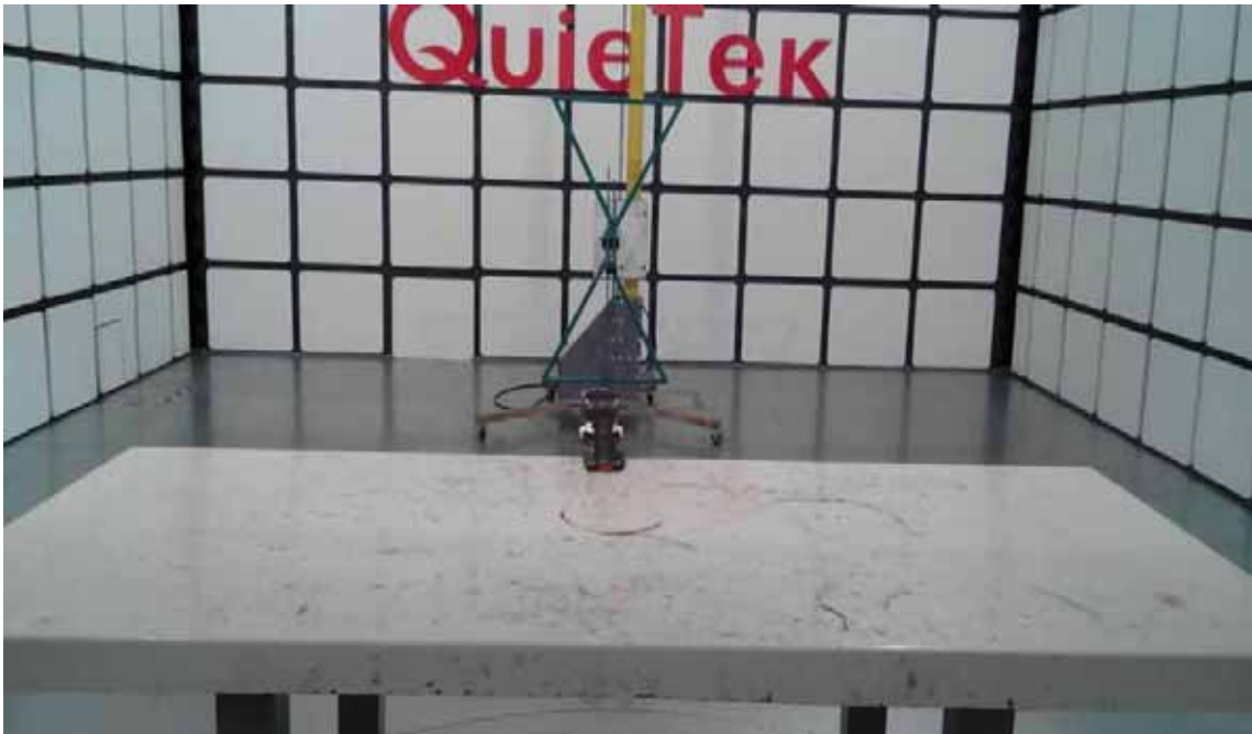
Description: Radiated Emission Test Setup for Below 1GHz
