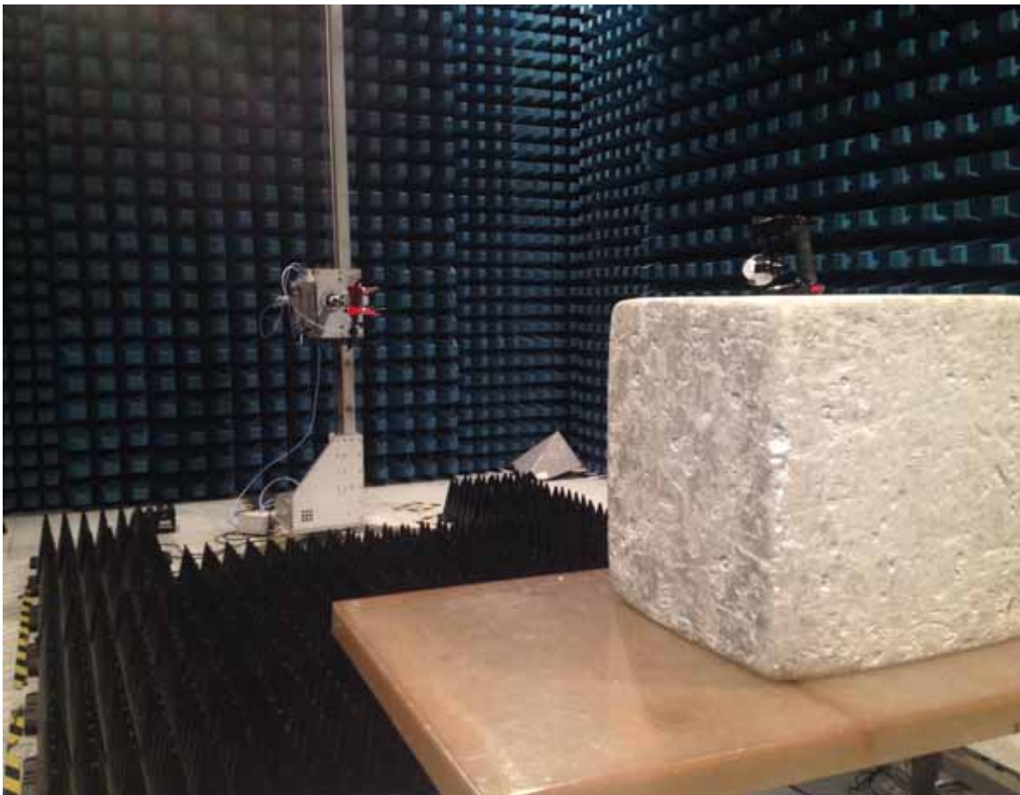
Description: Radiated Emission Test Setup for 1~18GHz
