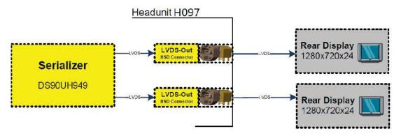
Yellow parts are not assembled in the production of H087
