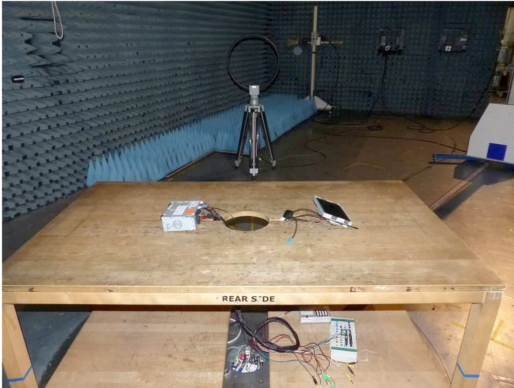
Photo 1: Test setup for radiated measurements (below 30 MHz)
