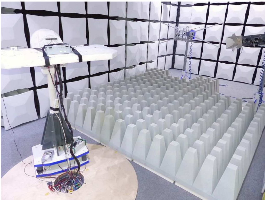
Photo 3: Test setup for radiated measurements (above 1 GHz)
