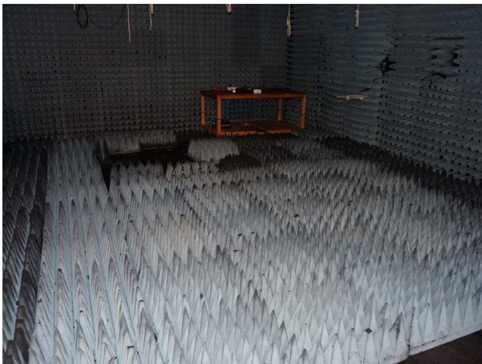
Photo 1,2: Test setup for radiated measurements, EUT in horizontal position Enclosure, semi-anechoic chamber, below 30 MHz, intentional radiator §15
