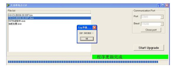
**4**) After finishing the upgrading, upper computer software will pop-up a dialog box to remind you of upgrading successfully, radio modem resetting, digital tube show bright, which means you upgrade successfully.
