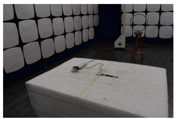
3. Radiated emission (9KHz-30MHz)
