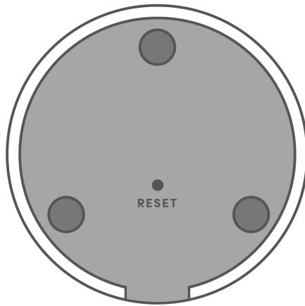
If, for any reason, you must perform a factory reset, you need to press and hold the pinhole button for between 10-15 seconds. Note that all your account settings will be lost and the Hub Mini will return to factory default.
