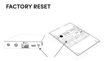
If, for any reason, you must perform a factory reset you need to press the pinhole button for between 10-15 seconds.
