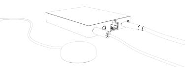
Connect your Flic IR accessory to the Hub via the 2.5mm connector and place the IR blaster in general the direction of the recieving device(s).
