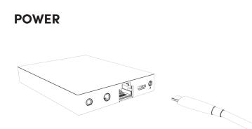
Connect the Micro USB cable to the Hub and an external power adapter. The Hub will now turn on, indicated by a bright red LED.
