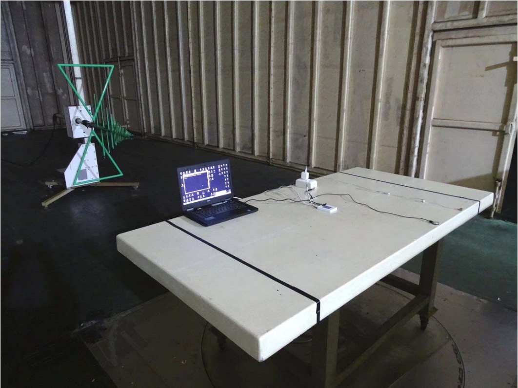
Front View of Radiated Test
