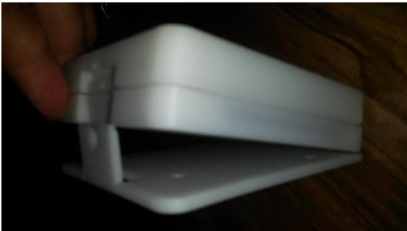
Figure 2: Tilt device forward then lift to remove from mount
