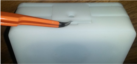
Figure 1: Lift wall mount tab using small pry tool
