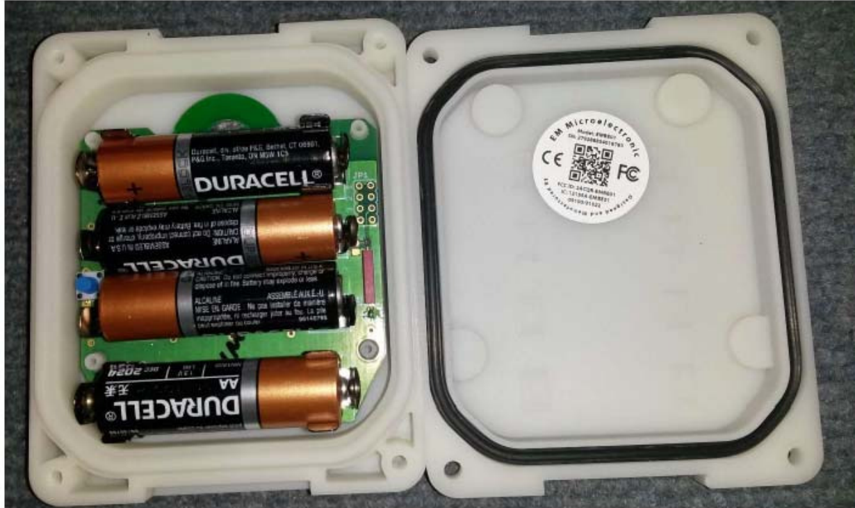
Enclosure Open Viewing Batteries.
