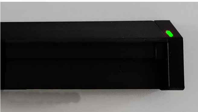
Figure 9 - After connecting the Battery Pack, the LED of the Rail Controller flashes 3x times in green colour (subject to change) during boot process
