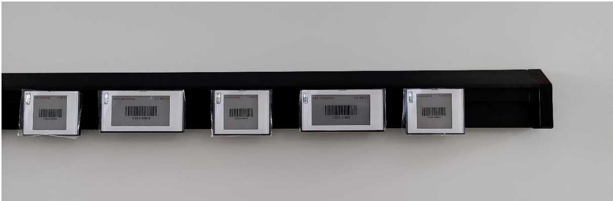
Figure 10 - Plugging Rail Displays into Rail
