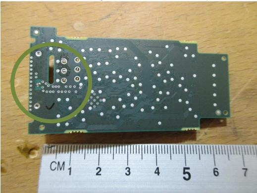
Bottom view of the PCB, antenna ground connection on the left and coplanar line:
