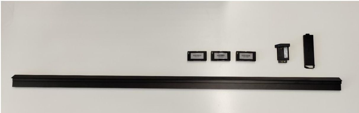
Figure 1 – Rail, Rail Controller, Battery Pack, Rail Displays
