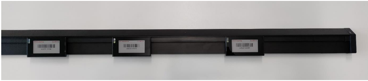
Figure 10 - Plugging Rail Displays into Rail
