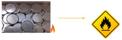
Lithium button batteries should NEVER be stored in contact with each other and without sufficient protection.
