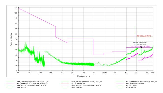
Worst case Emission: 53,4 dB $\mu$ V/m Peak at 4808 MHz equals to 27,3 dB $\mu$ V/m Average calculated with the factor described on page 8 of this test report.
