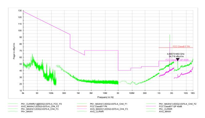
Worst case Emission:  $54.7 \text{ dB}\mu\text{V/m}$  Peak at 4808 MHz equals to  $28.6 \text{ dB}\mu\text{V/m}$  Average calculated with the factor described on page 8 of this test report.
