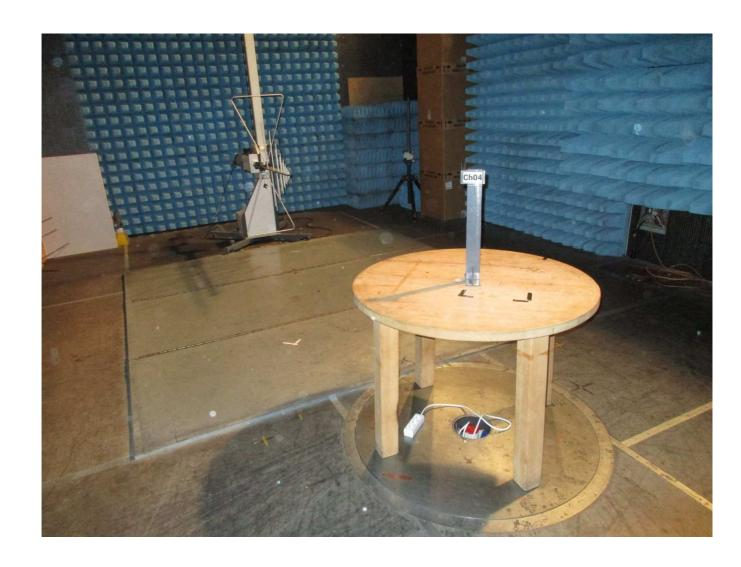
Description: Test setup above 1 GHz
