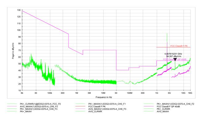
Worst case Emission: 54,4 dB $\mu$ V/m Peak at 4808 MHz equals to 28,3 dB $\mu$ V/m Average calculated with the factor described on page 8 of this test report.
