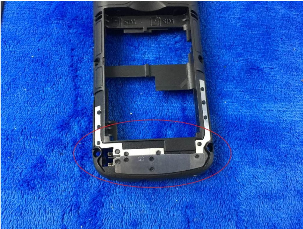
GSM/PCS Antenna View
