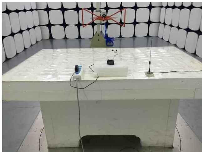
Conducted Emissions Test Setup Front View
