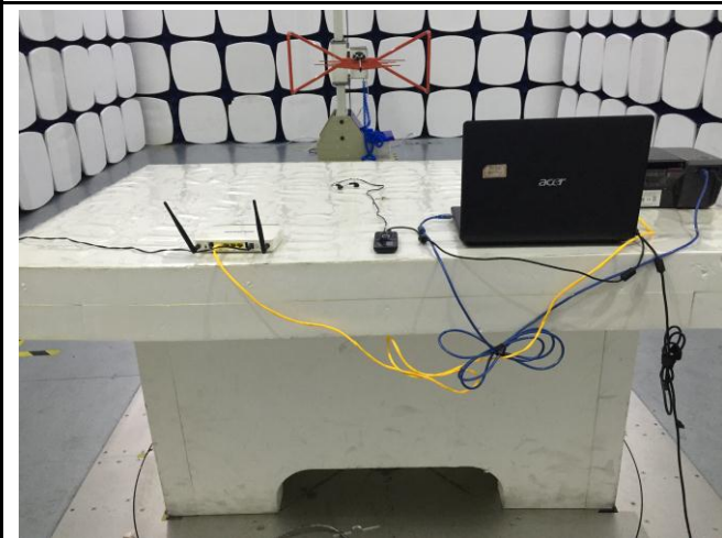
Radiated Emissions Test Setup Below 1GHz
