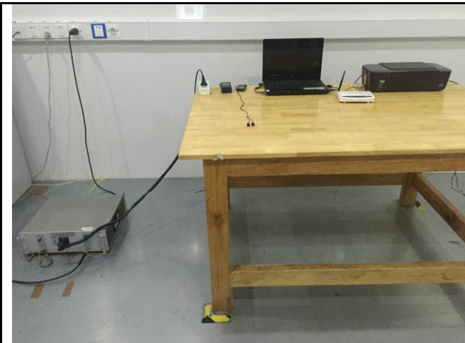
Conducted Emissions Test Setup – Front View
