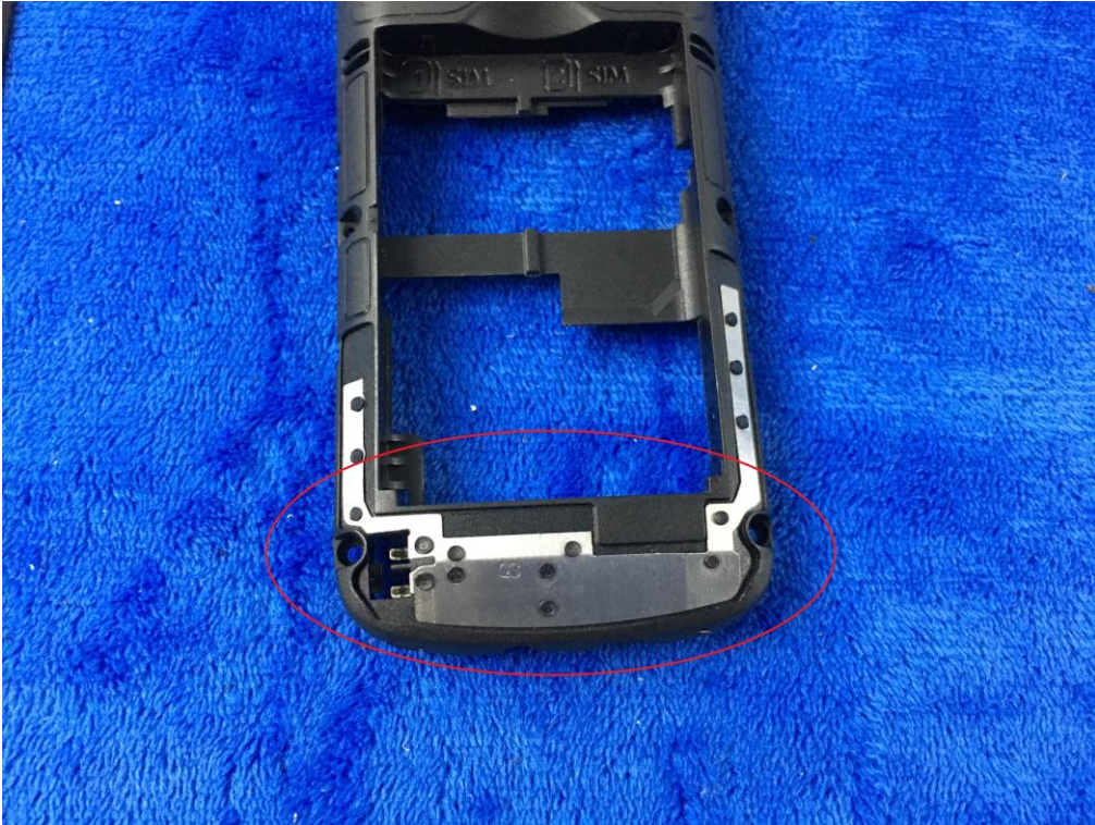
GSM/PCS Antenna View
