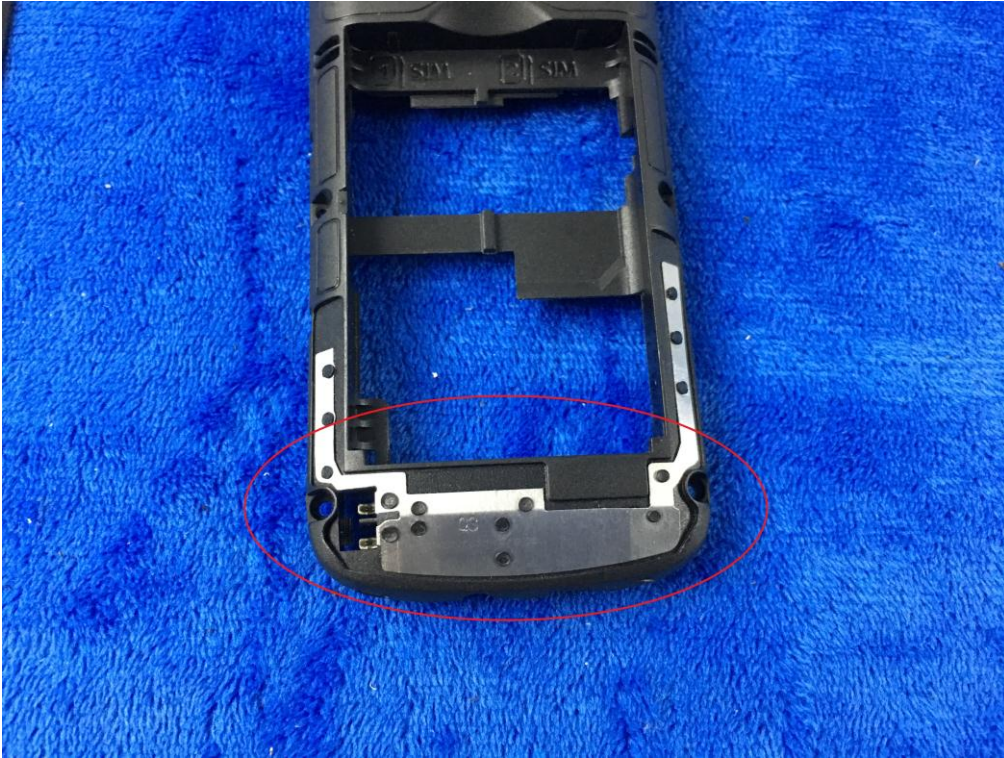
GSM/PCS Antenna View
