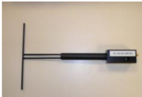
Figure 1 – Satimo COMOSAR Validation Dipole
