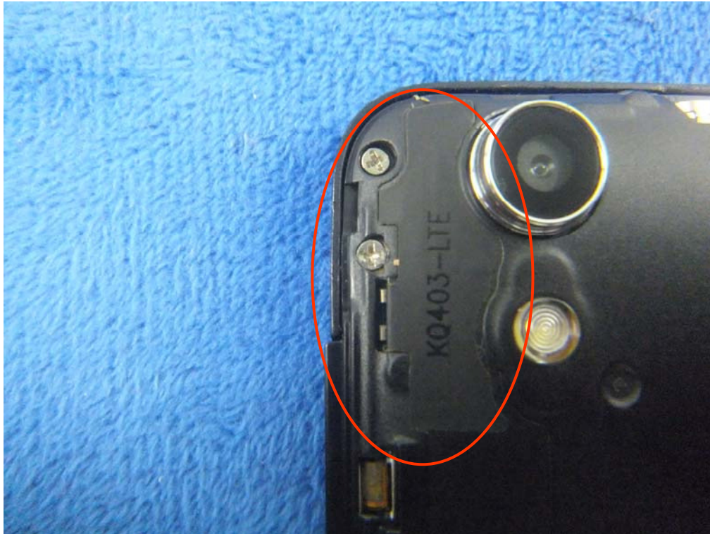
LTE - Antenna View
