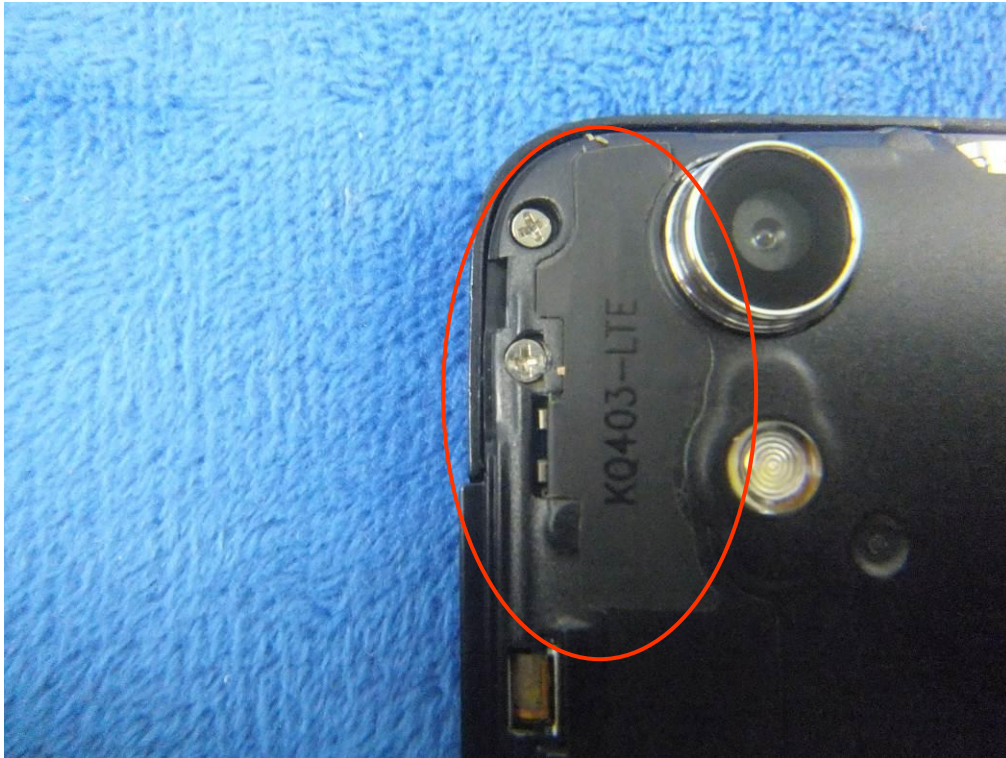
LTE - Antenna View
