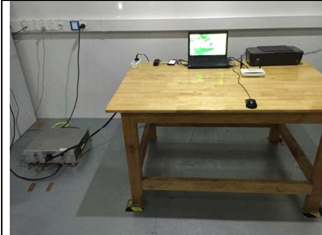
Conducted Emissions Test Setup – Front View
