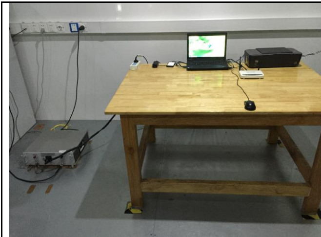
Conducted Emissions Test Setup – Front View
