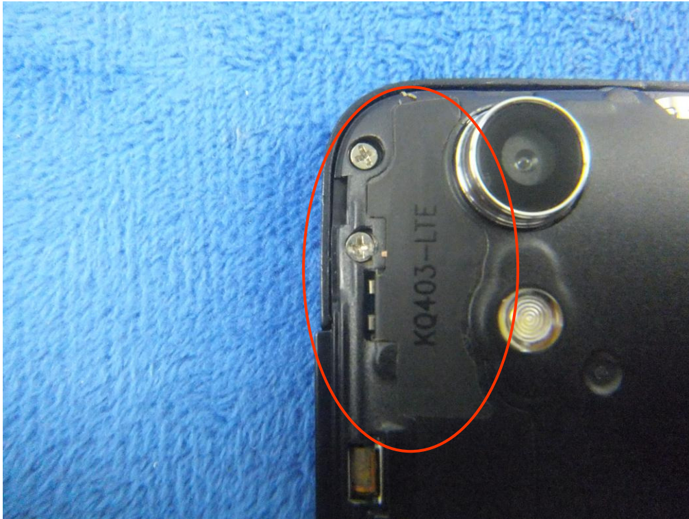
LTE - Antenna View
