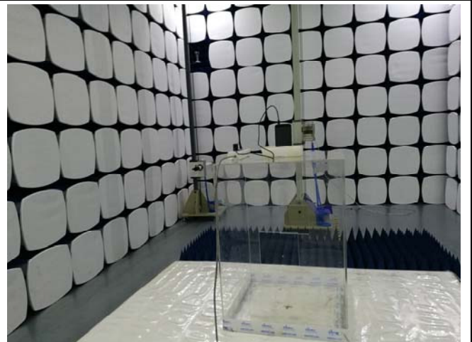
Radiated Spurious Emissions Test Setup Above 1GHz
