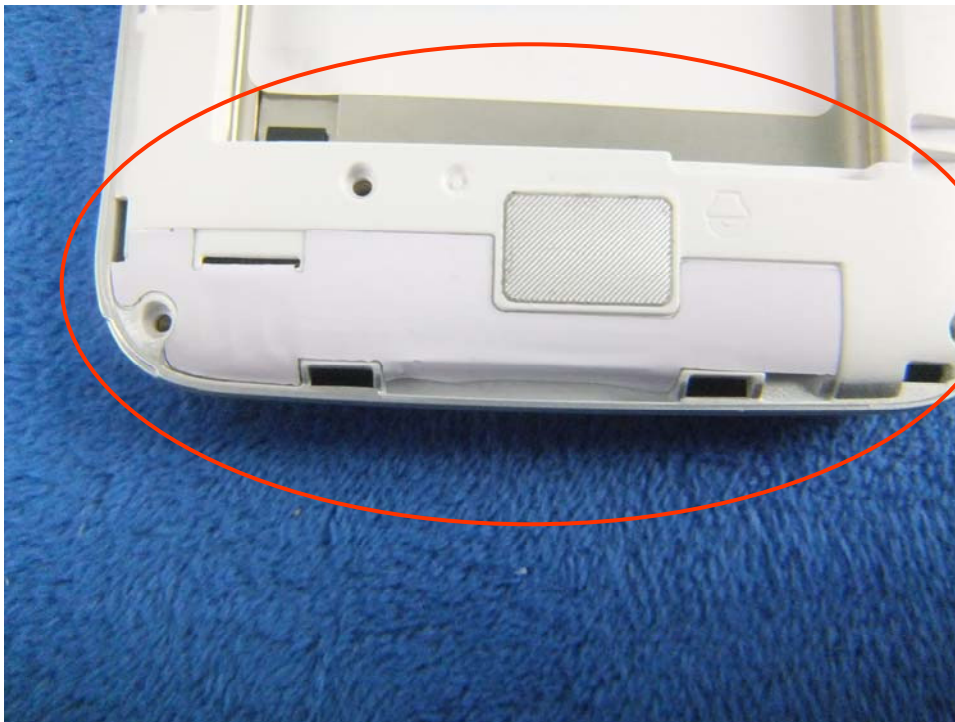
GSM/PCS/UMTS - Antenna View
