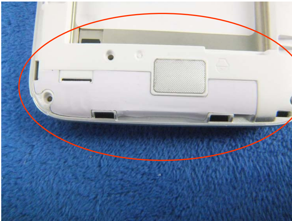
GSM/PCS/UMTS - Antenna View
