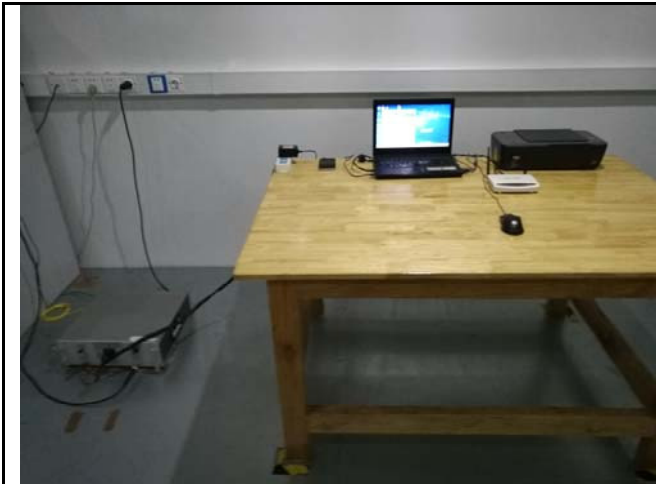
Conducted Emissions Test Setup – Front View
