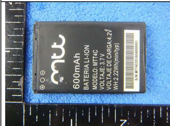
Battery - Front View
