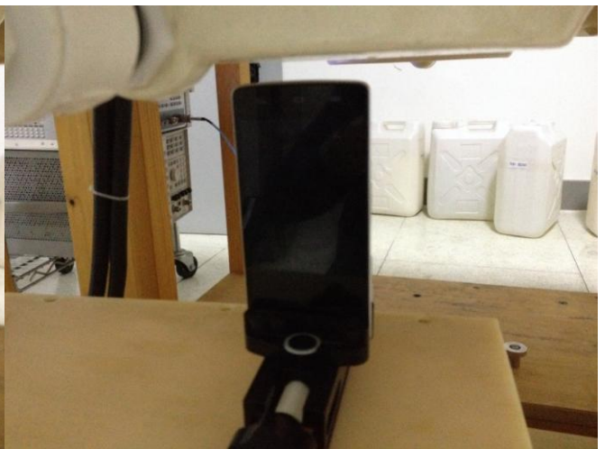
Bottom of the EUT with 1 cm Gap
