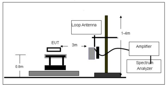
(B) Radiated Emission Test-Up Frequency 30MHz~1GHz
