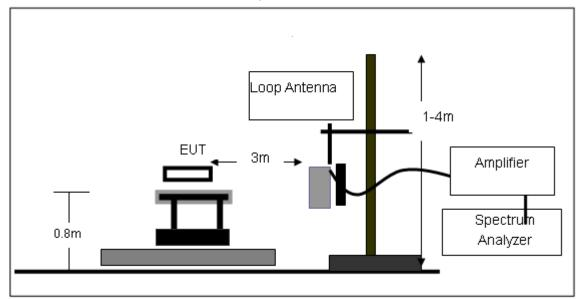
(B) Radiated Emission Test-Up Frequency 30MHz~1GHz
