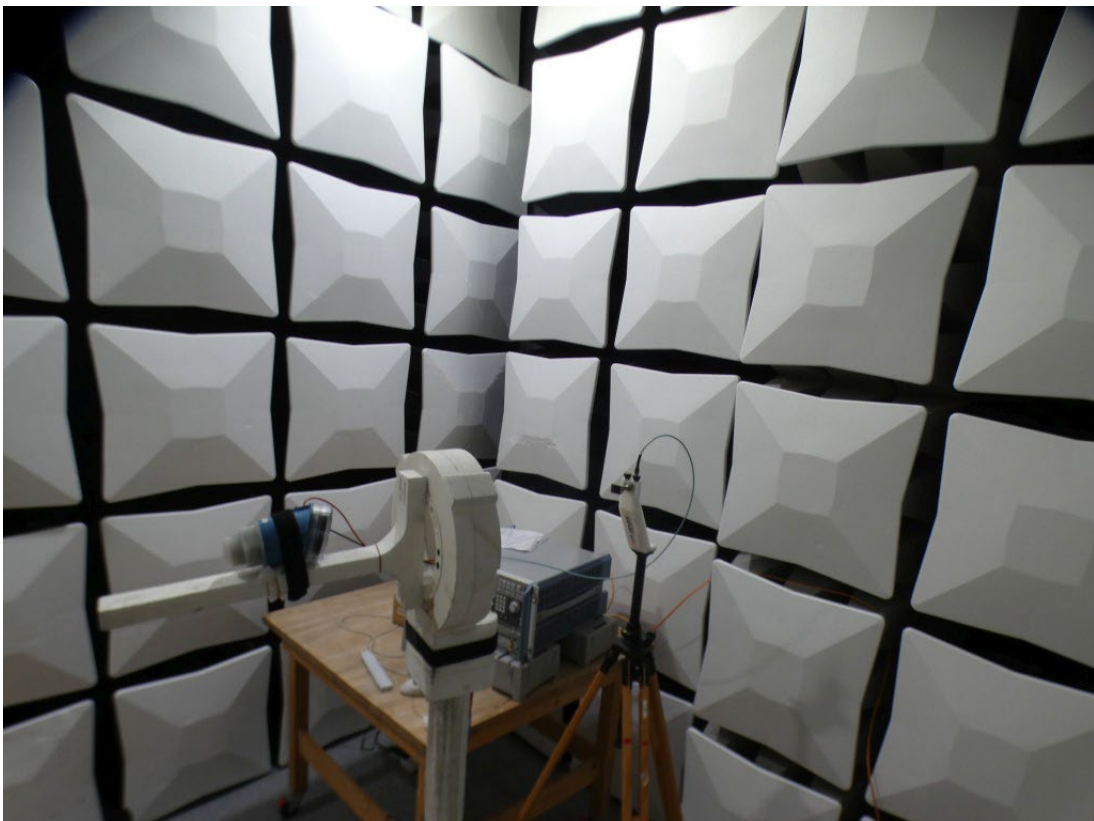
Photo 6: Test setup for radiated measurements above 26 GHz
