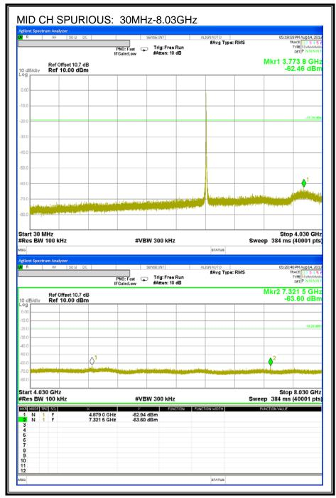
**Note**: Per 11.3 of KDB 558074 (v03r01), number of points must be >/= Span/RBW. Therefore, seven plots are needed to satisfy this requirement over the range of 30MHz-26GHz.
