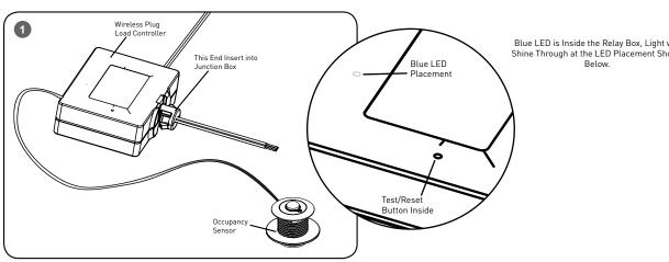
Blue LED is Inside the Relay Box, Light will Shine Through at the LED Placement Shown
