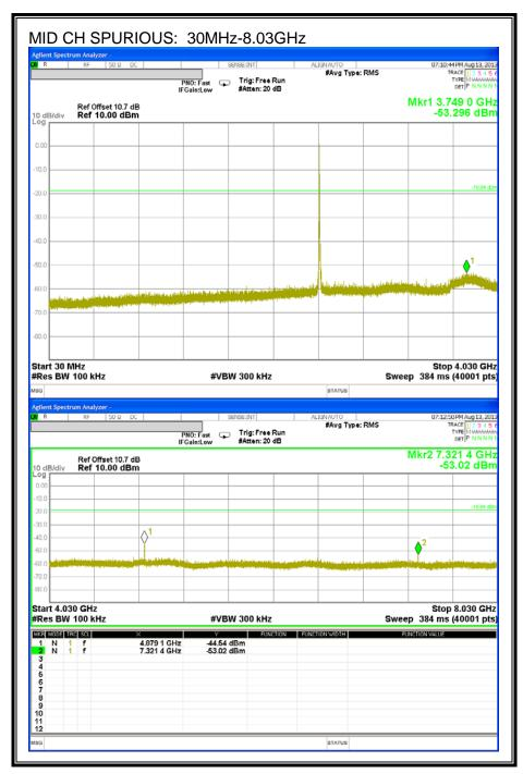
**Note**: Per KDB 558074, number of points must be >/= Span/RBW. Therefore, seven plots are needed to satisfy this requirement over the range of 30MHz-26GHz.
