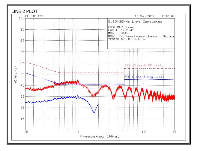
**Note:** Blue trace is a reduced video-bandwidth scan to determine presence of narrow-band emissions.
