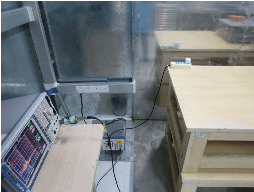
FCC RADIATED EMISSION TEST SETUP
