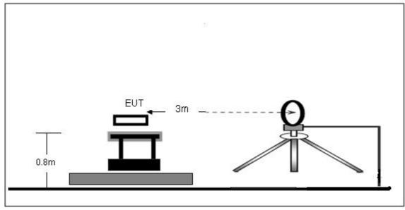
(B) Radiated Emission Test-Up Frequency 30MHz~1GHz
