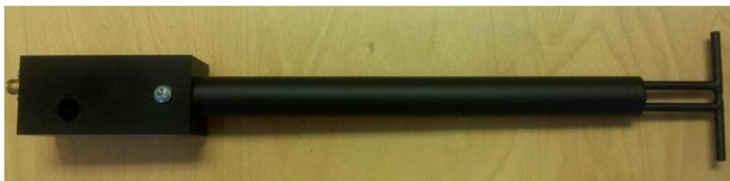
Figure 1 – MVG COMOSAR Validation Dipole
