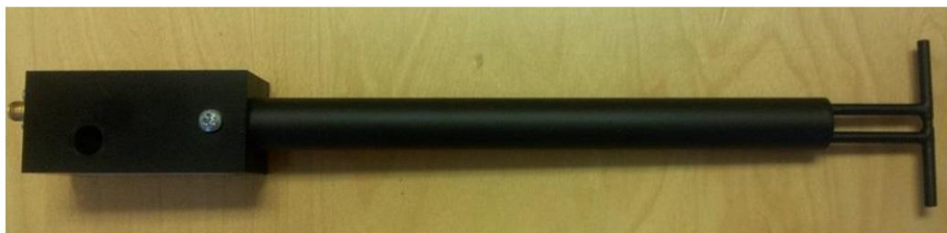
Figure 1 – MVG COMOSAR Validation Dipole
