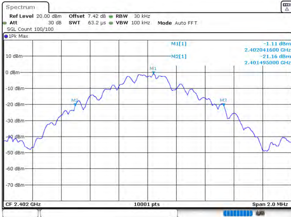
-20dB Bandwidth NVNT 1-DH5 2402MHz Ant1
