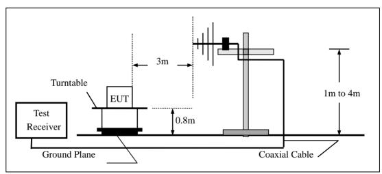
(c) For radiated emissions above 1000MHz
