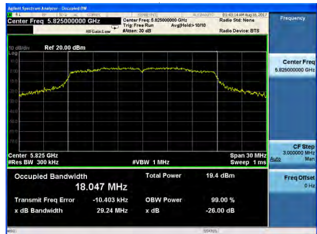
(802.11 AC20) -26dB&99%Bandwidth plot on channel 165
