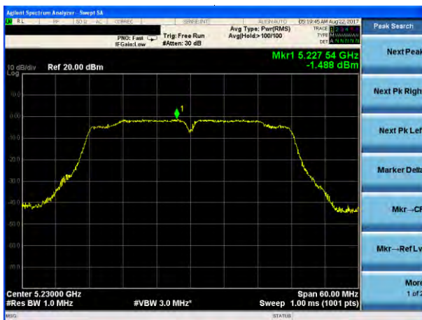
(802.11n40) PSD plot on channel 46
