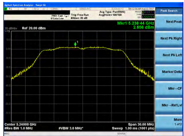
(802.11n20) PSD plot on channel 48
