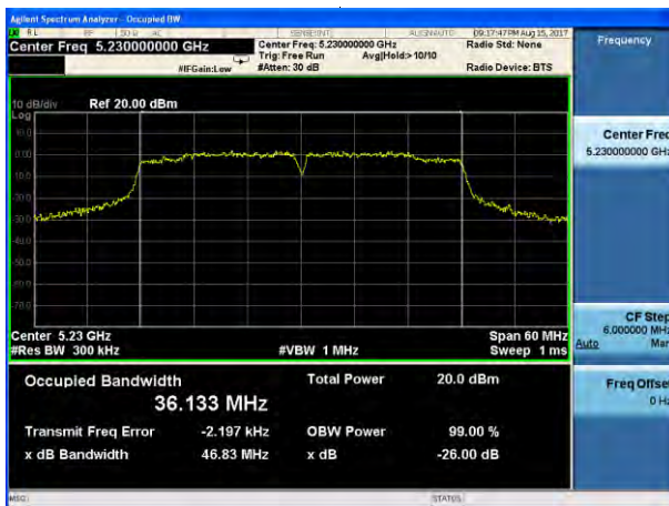
(802.11 n40) -26dB&99%Bandwidth plot on channel 46
