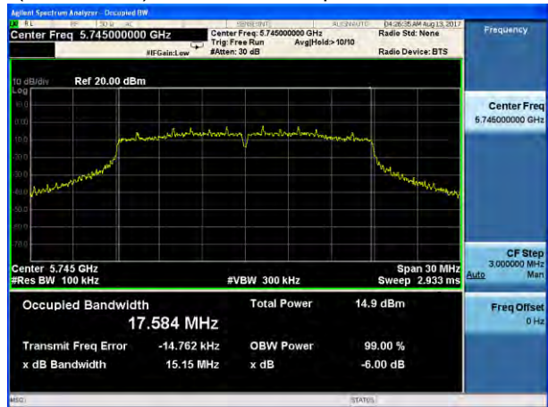
(802.11 n20) 6dB Bandwidth plot on channel 149
