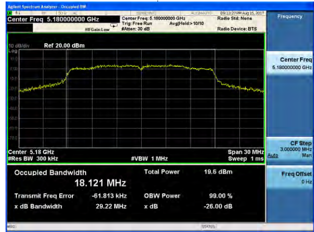
(802.11 AC20) -26dB&99%Bandwidth plot on channel 40
