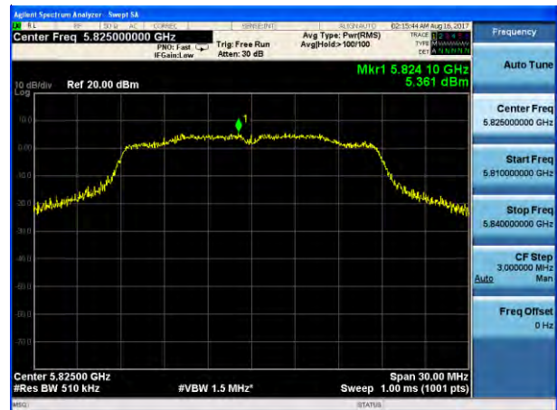
(802.11n20) PSD plot on channel 165
