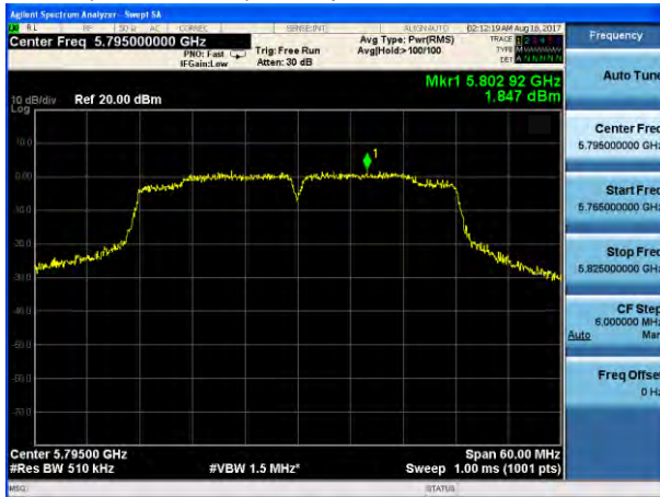
(802.11ac40) PSD plot on channel 159
