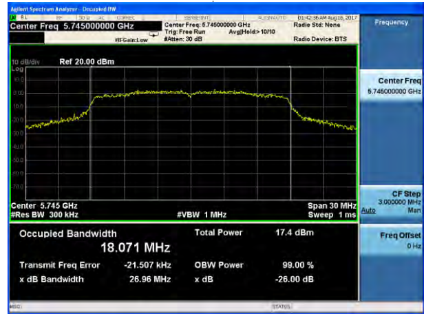
(802.11 AC20) -26dB&99%Bandwidth plot on channel 157
