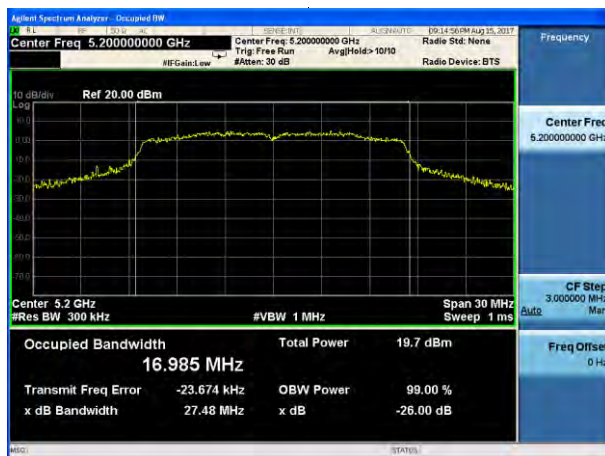
(802.11a) -26dB&99%Bandwidth plot on channel 48
