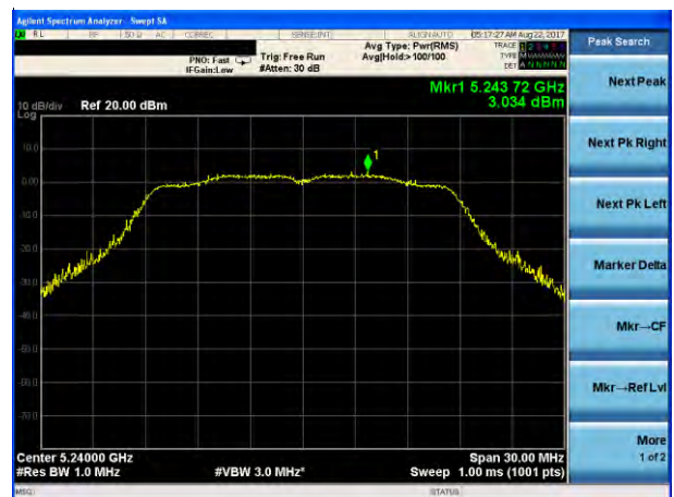
(802.11ac20) PSD plot on channel 48
