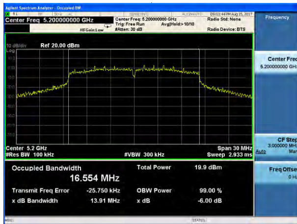
(802.11a) 6dB Bandwidth plot on channel 48
