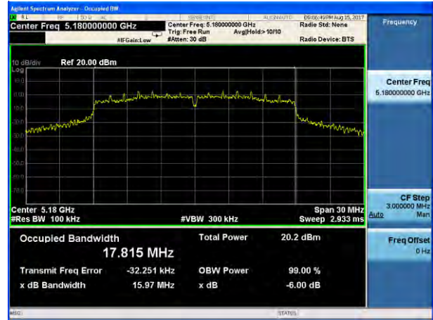
(802.11 n20) 6dB Bandwidth plot on channel 40
