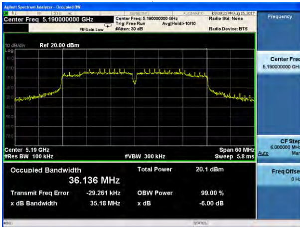
(802.11 AC40) 6dB Bandwidth plot on channel 46
