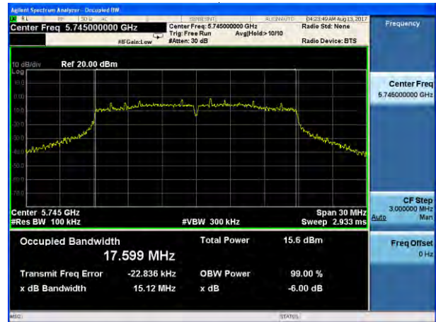
(802.11 AC20) 6dB Bandwidth plot on channel 157
