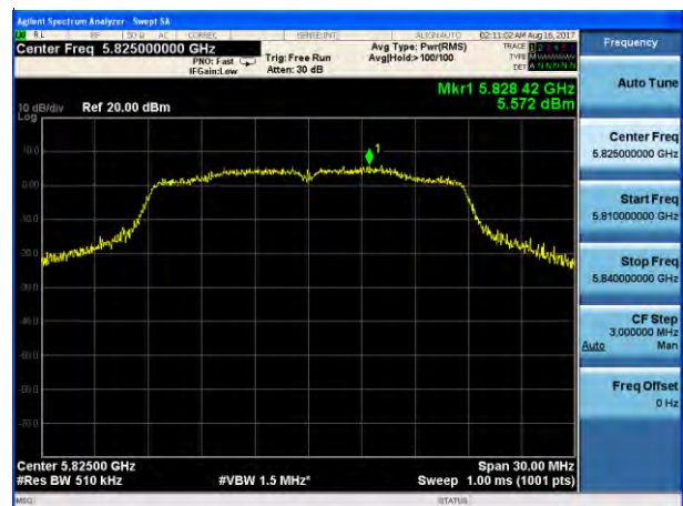
(802.11ac20) PSD plot on channel 165
