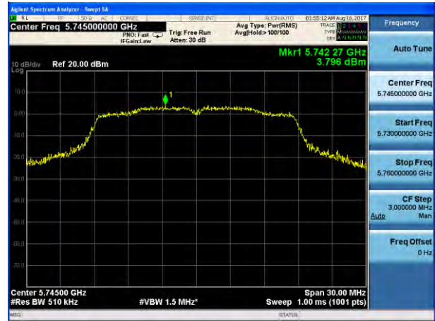
(802.11ac20) PSD plot on channel 157
