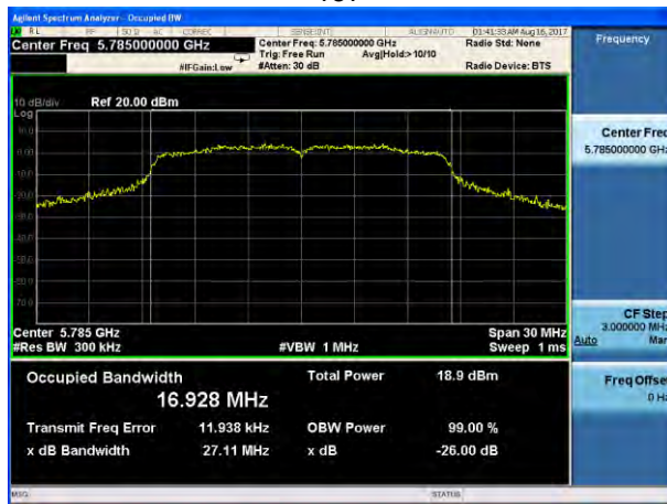
(802.11a) -26dB&99%Bandwidth plot on channel 157
