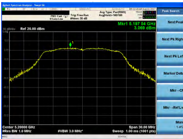
(802.11a) PSD plot on channel 48
