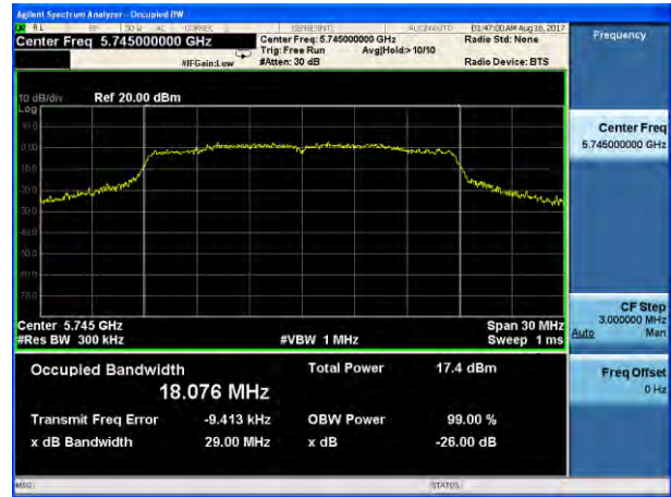
(802.11 n20) -26dB&99%Bandwidth plot on channel 149
