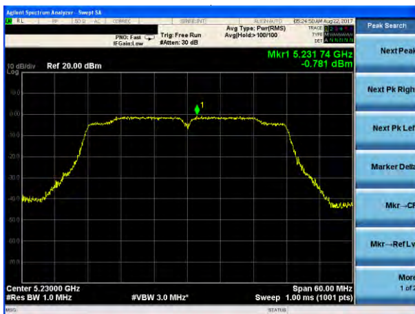
(802.11ac40) PSD plot on channel 46
